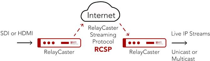
Using the RelayCaster Streaming Protocol (RCSP) as streaming protocol between two RelayCaster servers allows for the optimized transmission of live IP streams to remote company sites, data centers, or networks. Compared to streaming with UDP or RTP, RCSP greatly reduces packet loss. Compared to content distribution with TCP or higher-level protocols, such as FTP or HTTP, GMIT's RCSP offers much higher bandwidths for transmission of live content over lossy long distance links.
